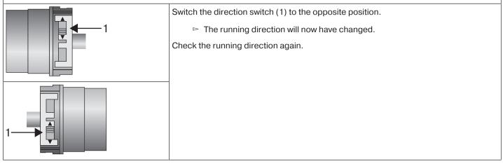
It is only possible to change the direction of rotation if no limit position has been set. It may be necessary to delete both limit positions in order to change the direction of rotation.
